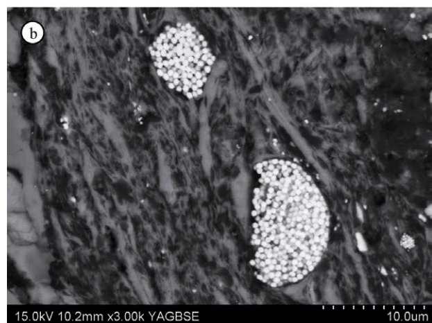
Figure 2. (a) Fractures in pyrite filled with chalcopyrite, bitumen and calcite; (b) framboidal pyrites in shale
