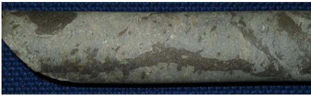
Figure 4. The nodules assemble into larger blobs of magnetite joining up into a network of ore veins. Kiirunavaara footwall.
