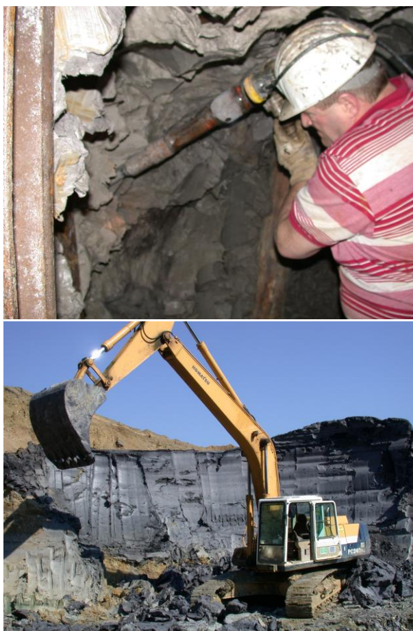
Figure 1. Top: Underground mining of pencil clay in the Klingenberg deposit, bottom: open pit mining of the Kärlich blue clay.
