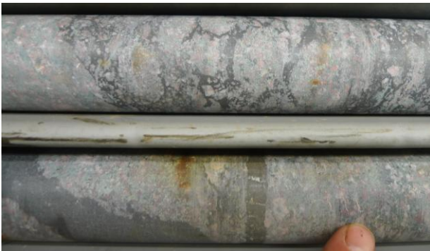
Figure 13. Variations in structural relation between ore veins and hanging wall porphyry; from intricate network of thin magnetite veins and rounded pieces of porphyry, and thicker vein with irregular contact, to relatively sharply cutting vein. Kiirunavaara hanging wall.
