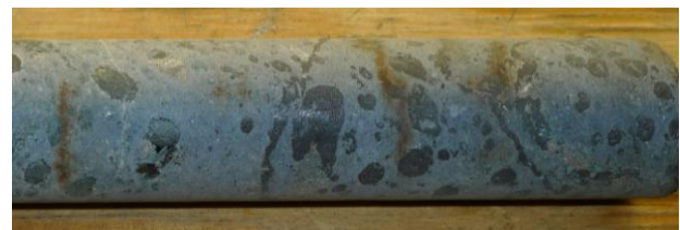
Figure 2. Magnetite-dominated nodules in Kiirunavaara footwall porphyry. The nodules are always rounded, but show variable forms, sizes and length-breadth ratios. Core diameter in all figures = 28 mm.
