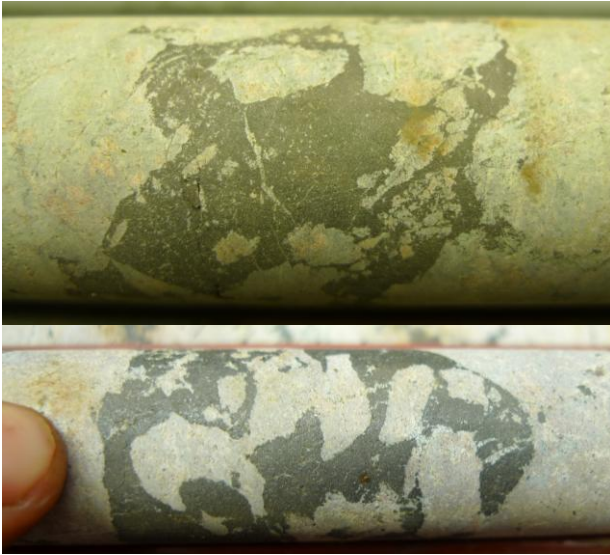
Figure 11. Two examples of irregular and rounded magnetite enclaves, carrying numerous smaller, more or less rounded inclusions of porphyry. Kiirunavaara hanging wall.
