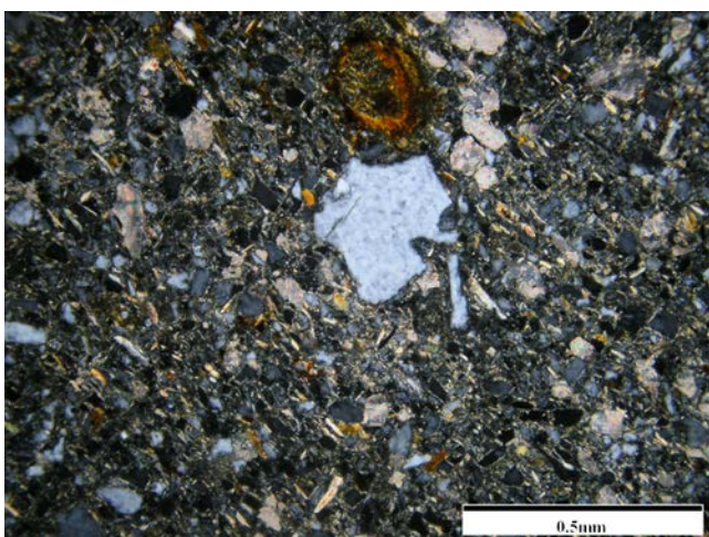
Figure 3. Microstructure of loess from Kunovice.
