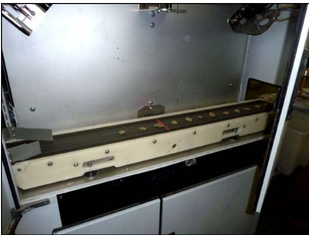
Figure 2. PetroScope® conveyor belt with optical cameras scanning individual grains
