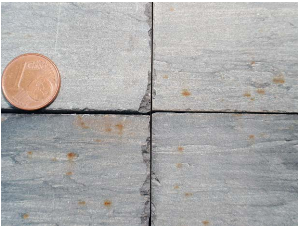
Figure 3. Resistance to ageing by thermal shock of XNFC. Surface detail of 3 tested specimens. Notice that the spots of iron oxide appeared mainly on the lighter colour levels. The specimen with coin on his top face is the reference specimen which was not submitted to testing.
