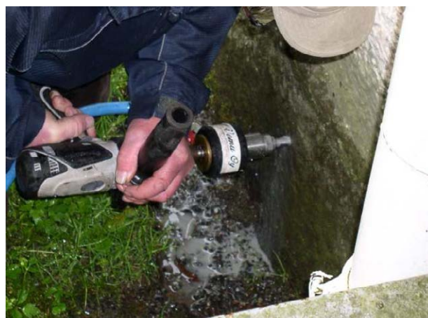
Figure 6. Sampling from a stone basement covered with moss. Photo Hannu Luodes.
