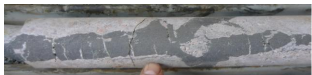
Figure 10. Typical example of small magnetite vein with irregular, bulbous contacts in the Kiirunavaara hanging wall porphyry. Calcite-filled, radial contraction fractures as seen here are typical for all magnetite veins and dykes. Kiirunavaara hanging wall.
