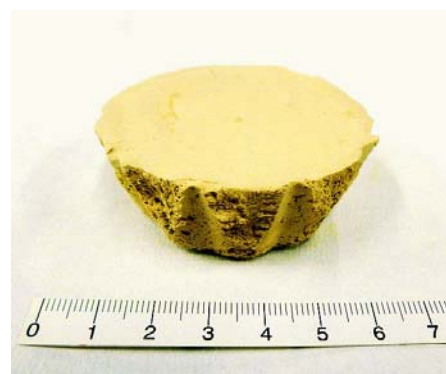
Figure 2. Sample of the Ecocement Block obtained mixing the CASO-urea bacterial culture with CKD.
