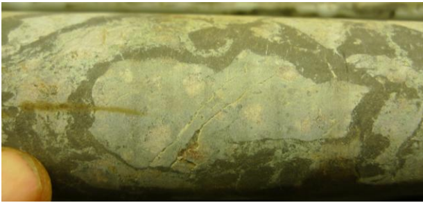
Figure 12. Irregular network of magnetite veins, intermingled with porphyry, showing rounded outlines. Kiirunavaara hanging wall.
