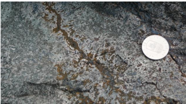
Figure 6. Magnetite-rich veins assembled in the nodule-rich footwall at Luossavaara. Diameter of coin = 25 mm.
