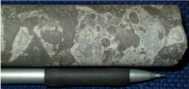
Figure 5. In places, the nodules are more or less completely engulfed in a chaotic mix of ore veins and remaining pieces of the nodular porphyry. Kiirunavaara footwall.
