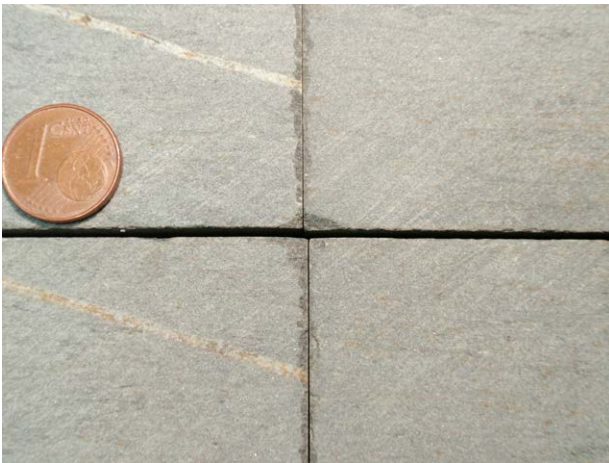
Figure 4. Resistance to ageing by thermal shock of XOFC. Surface detail of 3 tested specimens. Notice that the visual appearance of the tested specimens is similar to the reference specimen — specimen with coin on his top face — which was not submitted to testing.
