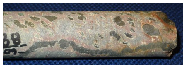
Figure 3. Commonly, the nodules are oriented in a flow-like or compaction pattern, and associated with a vein network. Kiirunavaara footwall.
