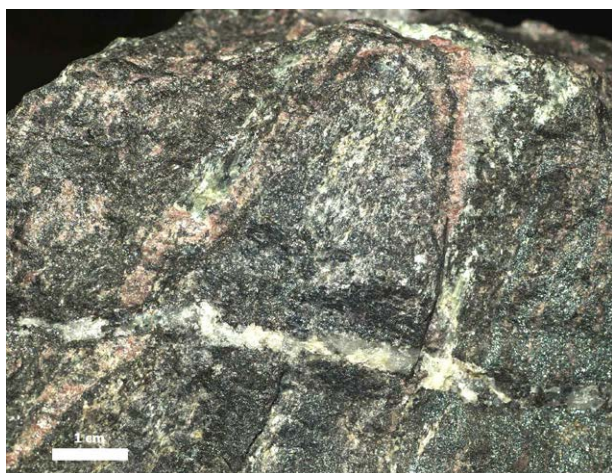
Figure 3. Hand-specimen scale folding of REE silicate bands in metamorphosed banded iron (BIF) ore at Högfors. Lighter cerite-(Ce)-dominated band is faulted and offset by a quartz vein (lower left). These veins carry additional allanite-type minerals. Scale bar equals 1 cm.
