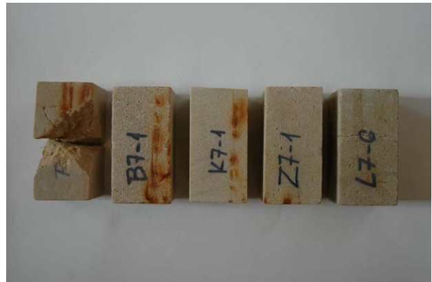
Figure 3. Studied sandstones after 120 freeze/thaw cycles. Rock types from the left: Hořice sandstone (P), Božanov sandstone (B), white variety of Kocbeře sandstone (K), yellow variety of Kocbeře sandstone (Z), Libná sandstone (L).
