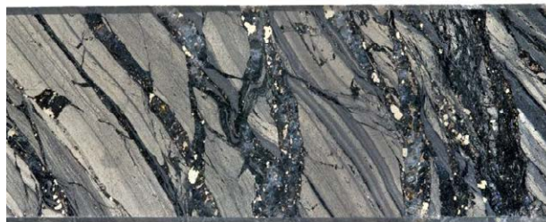
Figure 1. Metamorphosed sulphur-rich black shale from the Talvivaara Ni-Cu-Zn-Co deposit. The width of the drill core section is 3 cm and the sample length is 7 cm. The syndimentary/syndiagenetic laminae rich in pyrite and graphite are cut by quartz-sulphide veins.
