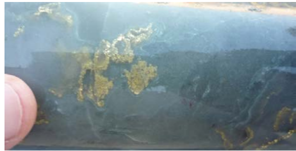
Figure 6. Electrum-rich bands containing fractal electrum dendrites from the Cambrian Haile, (SC) deposit, SE USA.
