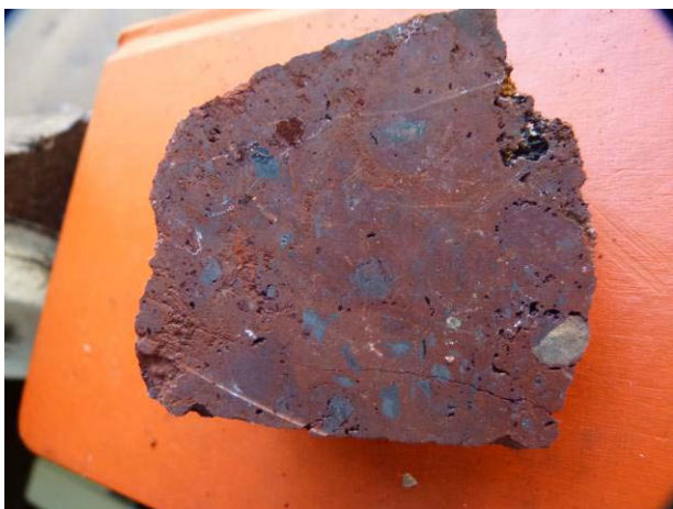
Figure 2. Replacement of the gossan (red) by siderite and galena (greyish) (“Red Rock”). Width of field: 15 cm.
