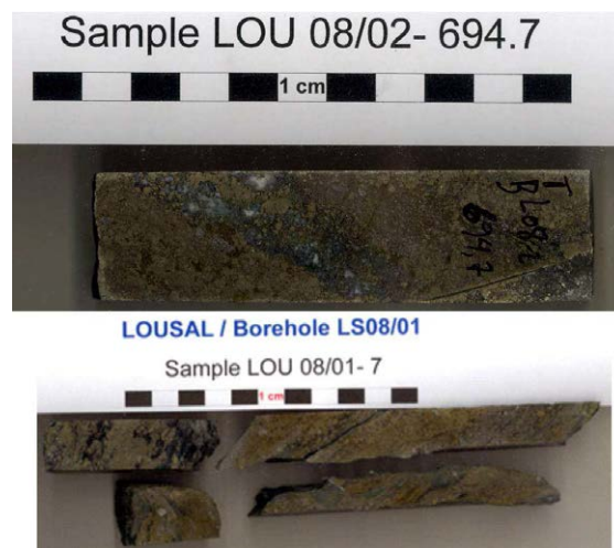
Figure 2. Hand specimen samples of gold-rich banded black shales with pyrite. The massive pyrite dominates the mineralogy at the hand specimen scale. (Borehole sample LOU 08/02 -694.7 upper photo; LOU08/01-7 lower photo).
