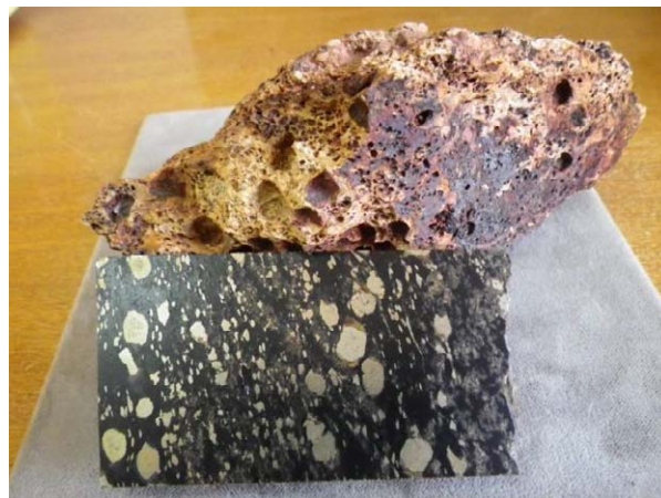
Figure 4. Lower part - magnetite rich meta-sediment containing large pyrite XX with chalcopyrite pressure shadows, pol. section. Upper part - the same rock type, but outcropping and strongly weathered, sample.
