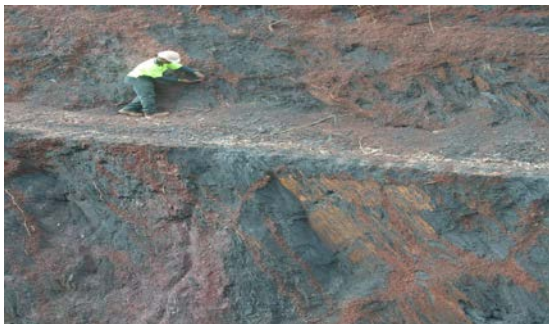
Figure 3: High grade enriched soft laminated (biscuity) supergene ore (Direct shipment Ore -DSO) at Mbalam. DSOs are limited or related to a very well defined plateau with deep soil and areas of laterite development.
