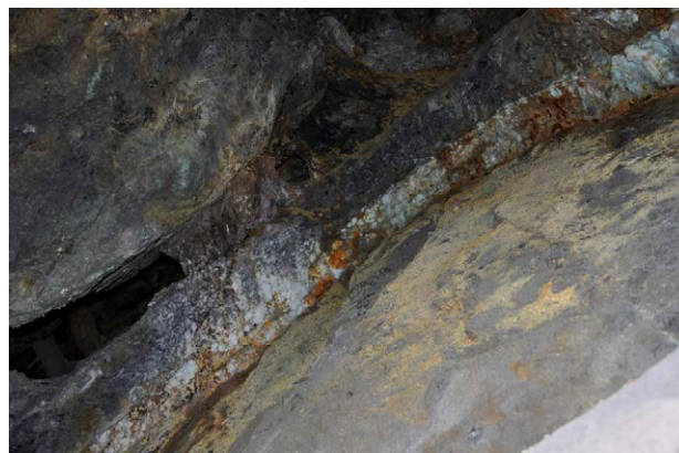
Figure 4. Evidences for multiphasic vein infilling in the veins of the Poopó fault system. The dark area is enriched in sphalerite and Sn sulphosalts and the clear area is filled by milky quartz. Total vein width is about 1,5 m.
