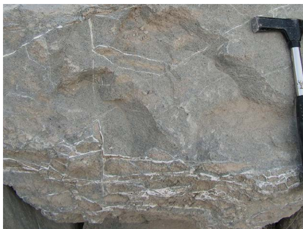
Figure 2. Alteration is most obvious along white natrolite veins and open mineralized fractures. The grayish rock matrix is also highly affected by zeolitization
