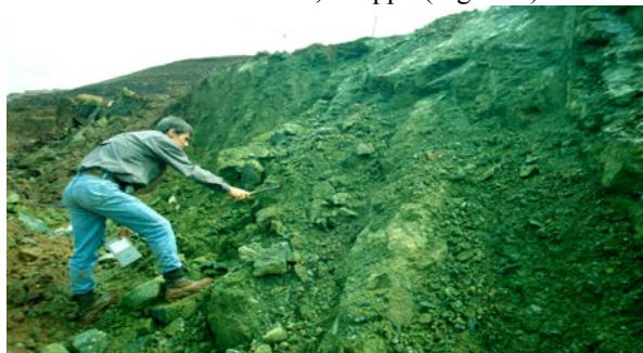
Figure 3. Sampling of Ni-laterites exposed in the open pit of the Corriola Mine, Niquelandia. The cude ore, mostly garnierite, contains up to 7.6 % Ni.
