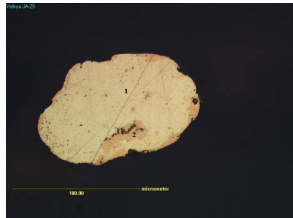
Figure 5. A zoned gold grain composed mainly of lighter Ag-Au alloy (point 1: 81.4 % Au, 18.5 % Ag) and partially rimmed by darker pure gold (99.4 % Au, 0.6 % Ag). The grain is separated from a crushed bulk rock sample from the discovery outcrop. Analysis from Kärkkäinen et al. (2012) appendix 1, sample JA-29Aconc./gr B/p1 and p2.
