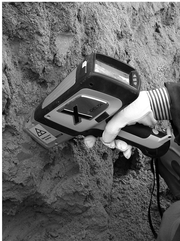
Figure 1. Portable XRF analysers can be used in mineral exploration due to its easy and fast usability in the field. Contents of the elements can be quickly analyzed even using natural till samples in fresh walls of the test pits. Photo by P. Sarala.
