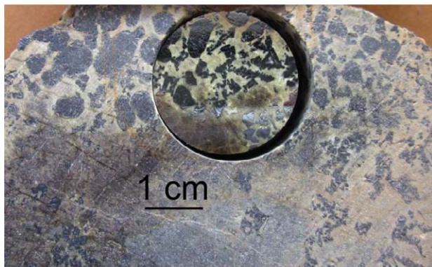
Figure 1. Skeletal crystals located between and on the edge of a group of chromite nodules.
