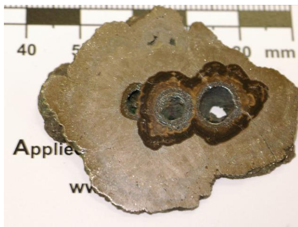
Figure 2. Cross section through the sulphide stalactite from Bolesław Mine with well visible internal channels in fibrous sphalerite and galena. The outer part is composed of banded pyrite and marcasite.
