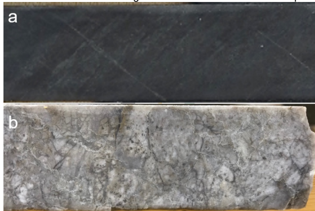
Figure 3. a. Least-altered coherent dacite surrounding the deposit DDC AKULL809, 140m depth. b. strongly altered in situ brecciated dacite displaying perlitic fractures from the central dacitic body DDC AKULL869, 177m depth.
