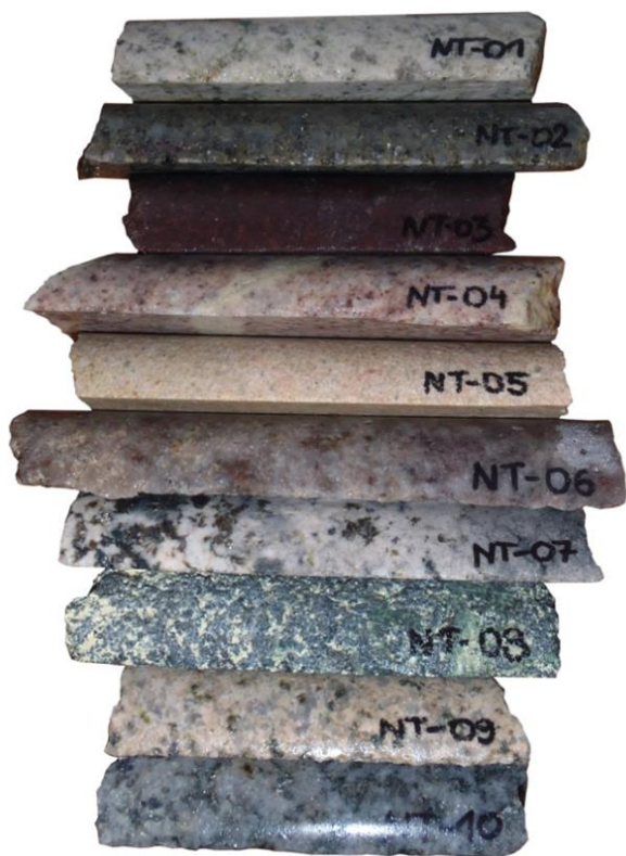
Figure 2. Mineralogical and petrographic variability of granites and greisens from Cínovec drill core (scale: half core sample NT-06 is 10 cm long).
