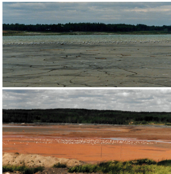
Figure 1. Pyrrhotite-bearing Au tailings in northwestern Ontario, Canada following deposition (top) and after one year of weathering (bottom).
