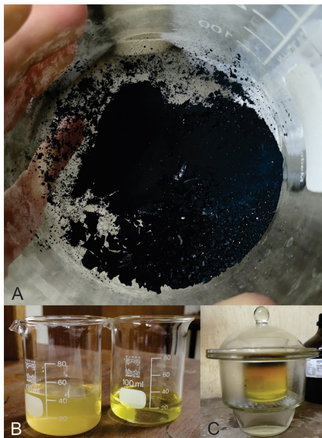
Figure 2. a. Prussian blue fine-grained crystals produced from rapid mixing of two solutions (potassium ferrocyanide and ferric chloride). b. Two solutions used for the single crystal grow. 7.5 mmol solution of \text{FeCl}_2 \cdot 3/4\text{H}_2\text{O} along with 2.5 mmol \text{K}_3[\text{Fe}(\text{CN})_6] . c. The 10 mol of HCl/L solution in a desiccator containing water.
