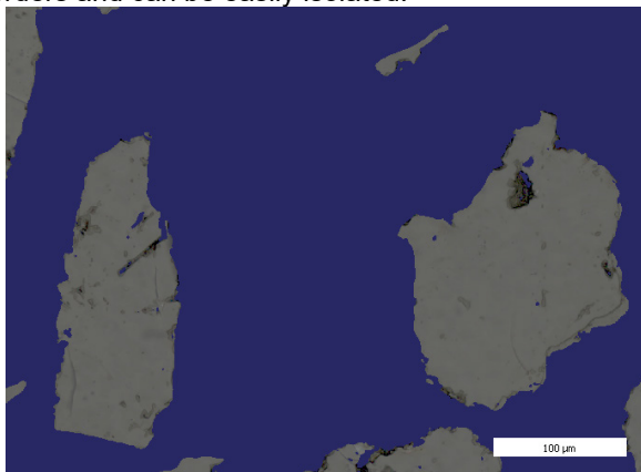
Figure 8. Mask for resin computed from image of Figure 6
