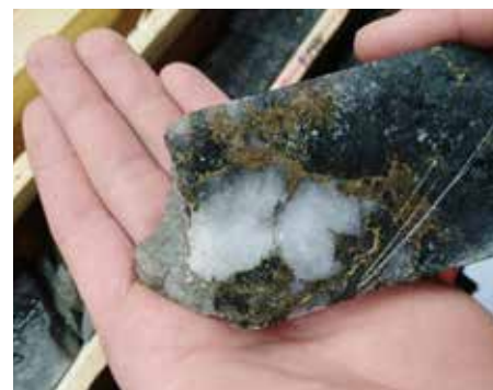
Figure 5. Sulfides (mainly pyrrhotite and chalcopyrite), typical example of ore hosting assemblage in the Portimo complex, with quartz clasts. Photo by K. Foltyn.
