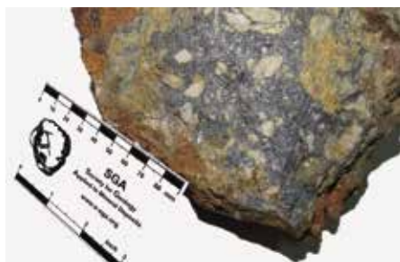
Figure 6. An example of breccia stibnite ore from the shear zone hosted Rizana deposit. Photo by K. Foltyn.
