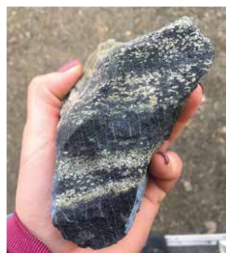
Fig. 7: Layered chromite ore.
