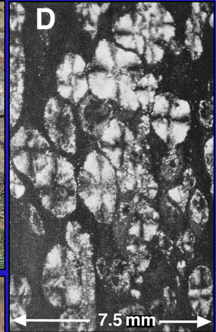
D. Barite in shale: packed spheroids of crystals grown radially on a core (Kraume et al. 1955)
